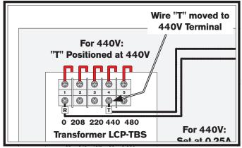
Figure 56. Wire "T" moved to 440V.
